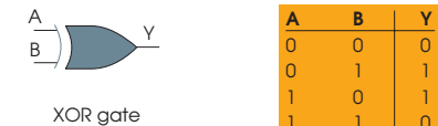
Figure 7-21. Boolean expression, gate symbol, and truth table for an XOR logic gate.
