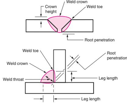
Figure 6-16. Weld and weld area terms.
