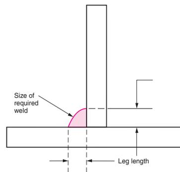
Figure 6-29. Fillet weld leg lengths from the root of the joint should be equal. Unequal leg length, unless otherwise specified, will not carry the designed load and may fail under stress.
