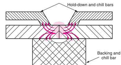
Figure 6-38. Tooling and bars used to remove heat from the weld and resist heat flow into the base material are sometimes called "chill bars."
