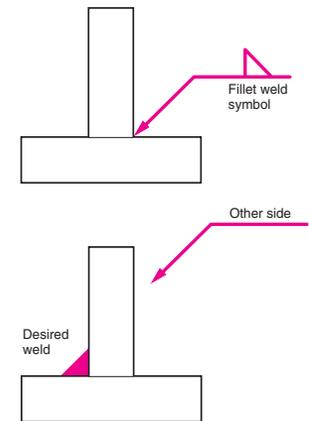
Figure 6-20. Fillet weld symbol shown on the upper side of the reference line indicates that the weld is located on the opposite side of the joint.
