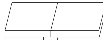
Figure 6-11. Plate butt weld with a fabricated backing bar.
