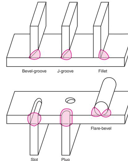
Figure 6-3. Types of welds that may be made with a basic T-joint.
