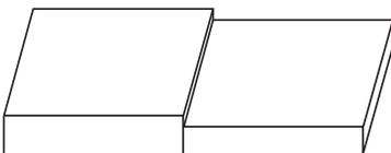
Figure 6-24. Mating the joint at the bottom equalizes the load during stress when the weld is made from the top and penetrates completely through the joint.
