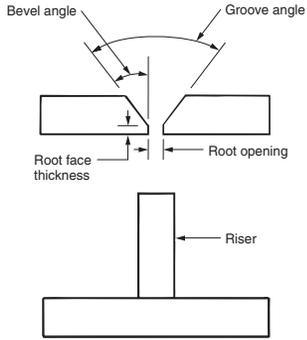
Figure 6-15. Weld joint terms.
