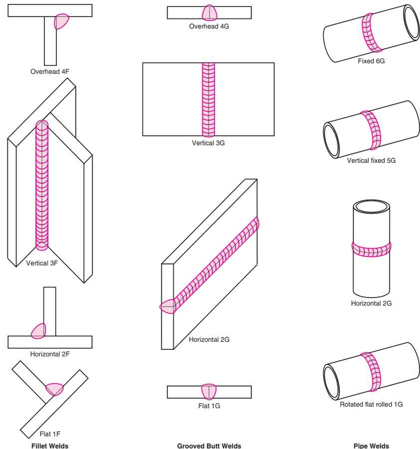
Figure 6-22. American Welding Society definitions of welding positions.
