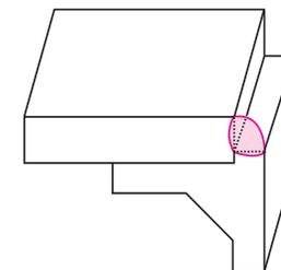
Figure 6-12. Controlled weld penetration joint.
