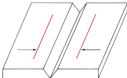
Figure 6-27. Weld joint shrinkage can be determined in four steps. 1. Tack weld the test joint together. 2. Scribe parallel lines, as shown, on approximately 2" centers. Record this dimension. 3. Weld joint with test weld procedure. 4. Measure linear distance and compare with original dimension.
