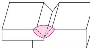
Figure 6-9. Tubular butt joint with a built-in backing bar.
