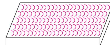
Figure 6-14. Overlaid welds, called surfacing or cladding, protect the base metal from wear or contamination.
