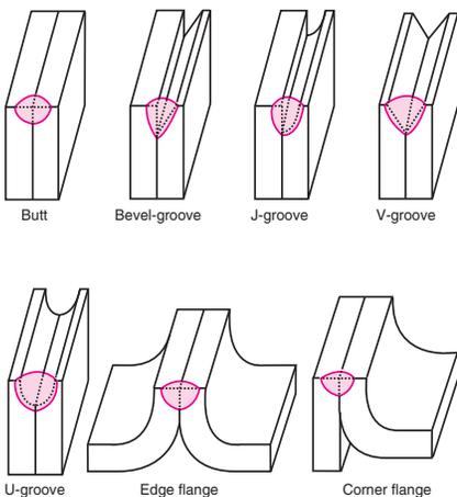
Figure 6-6. Types of welds that may be made with a basic edge joint.
