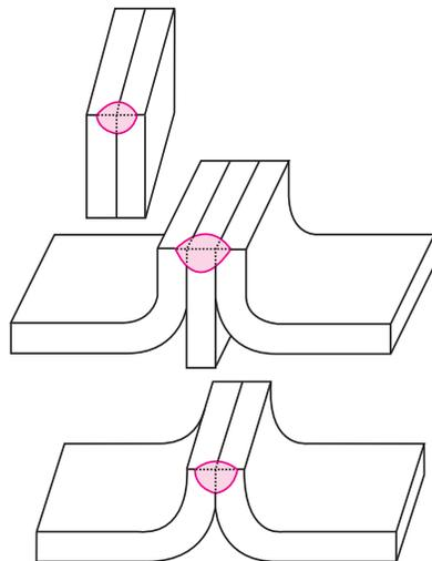
Figure 6-34. Common edge weld joint designs that may be used in fabrication.
