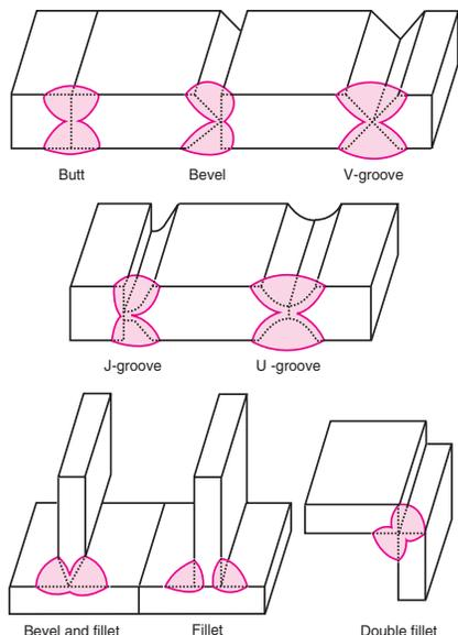
Figure 6-7. Applications of double welds.
