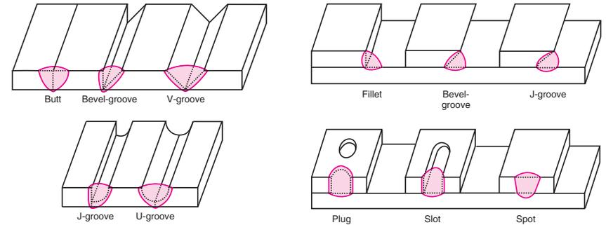
Figure 6-4. Types of welds that may be made with a basic lap joint.
