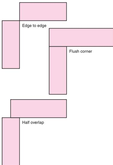
Figure 6-33. Common corner weld joint designs that may be used in fabrication.
