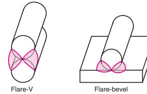
Figure 6-2. Types of welds that may be made with a basic butt joint.
