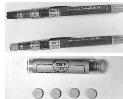
Figure 6-37. Temperature crayons and pellets may be used to determine preheating temperatures prior to welding.
