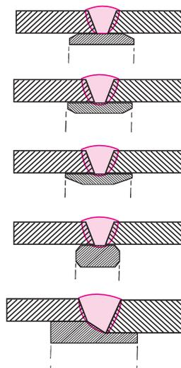
Figure 6-10. Various types of backing rings for pipe joints.
