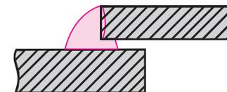
Figure 6-31. Lap joint problem areas that result from improper fit-up.
