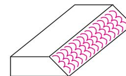
Figure 6-13. Buttered weld joint face.
