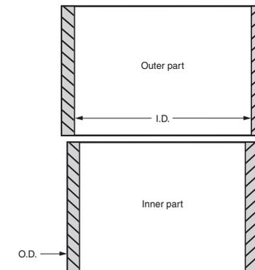
Figure 6-32. The diameters of the parts to be assembled with an interference fit may be found by using a "pi" tape around the inner and outer cylindrical components. The tape measures in thousandths of an inch and full inches.
