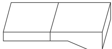
Figure 6-25. Joints of unequal thickness absorb different amounts of heat and expand at different ratios. Equalize the heat flow by tapering the heavier material to the thickness of the thinner material.
