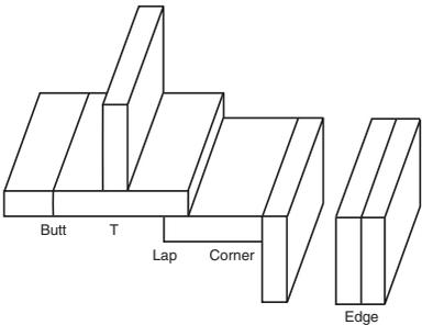
Figure 6-1. The five basic types of joints used in welding.
