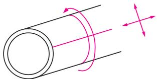
Figure 6-26. Butt welds shrink during welding in both transverse and circumferential directions.
