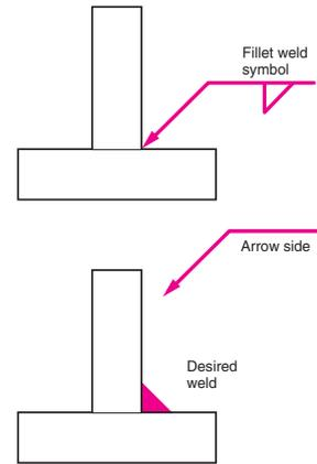
Figure 6-19. Fillet weld symbol shown on the bottom side of the reference line indicates that the weld is located where the arrow points.
