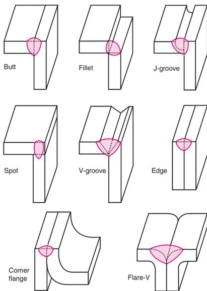
Figure 6-5. Types of welds that may be made with a basic corner joint.
