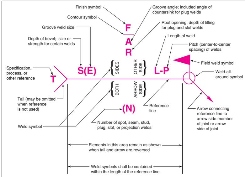
Figure 6-17. The AWS welding symbol conveys specific and complete information to the welder. (Printed with permission of the American Welding Society)
