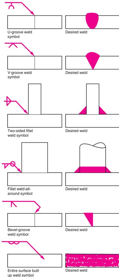
Figure 6-21. Typical weld symbols and weld applications.
