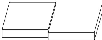
Figure 6-23. Welds made on mismatched joints often will fail below the rated load when placed in stress conditions.
