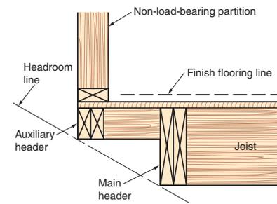
**Figure 18-7.** Extending the upper floor area with a shallow auxiliary header to provide headroom. The partition over the auxiliary header must not be load bearing.
