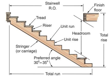
Figure 18-5. Basic stair parts and terms. The total number of risers is always one greater than the total number of treads.
