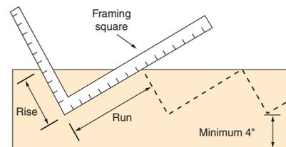
**Figure 18-14.** Using a framing square to lay out a stringer.
