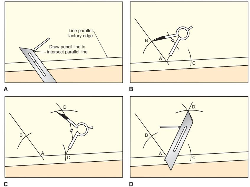
**Figure 18-24.** Splitting an angle for a miter cut. A—After drawing a line parallel to the factory edge, transfer the miter angle to the board. B—Draw arcs of equal lengths from the intersection of lines AB and AC. C—Swing arcs to create point D. D—Draw line AD. This is the miter angle.
