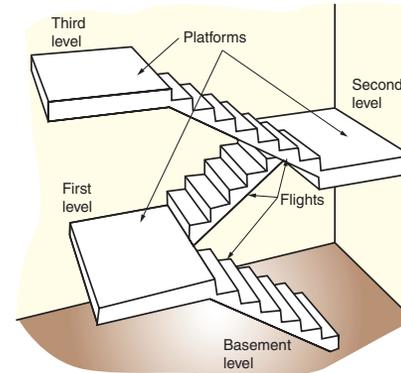
Figure 18-4. Stair runs are often made one above the other to gain headroom. This one is designed for a split-level home.
