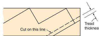
**Figure 18-16.** Trim the bottom end of the stringer to adjust the riser height for the tread thickness.
