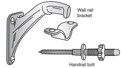
**Figure 18-30.** Hardware for stair rails. The handrail bolt is concealed in the center of a joint. The nut is accessible from below and can be adjusted with a screwdriver or a hammer and nail set.
