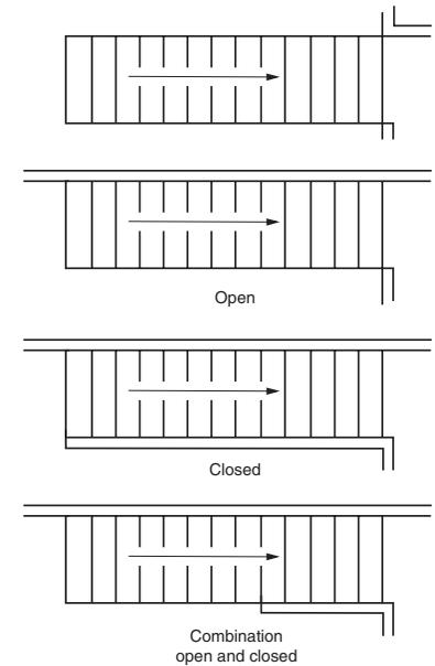
**Figure 18-2.** Open and closed stairways. A stair is called open even if one side is enclosed by a wall.
