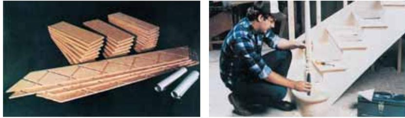
**Figure 18-28.** Prefabricated stairway system. A—Parts for the system. Stringer sections lock together with a common tread. B—This installed mock-up shows the assembled section mounted on substringers. (Visador Co.)
