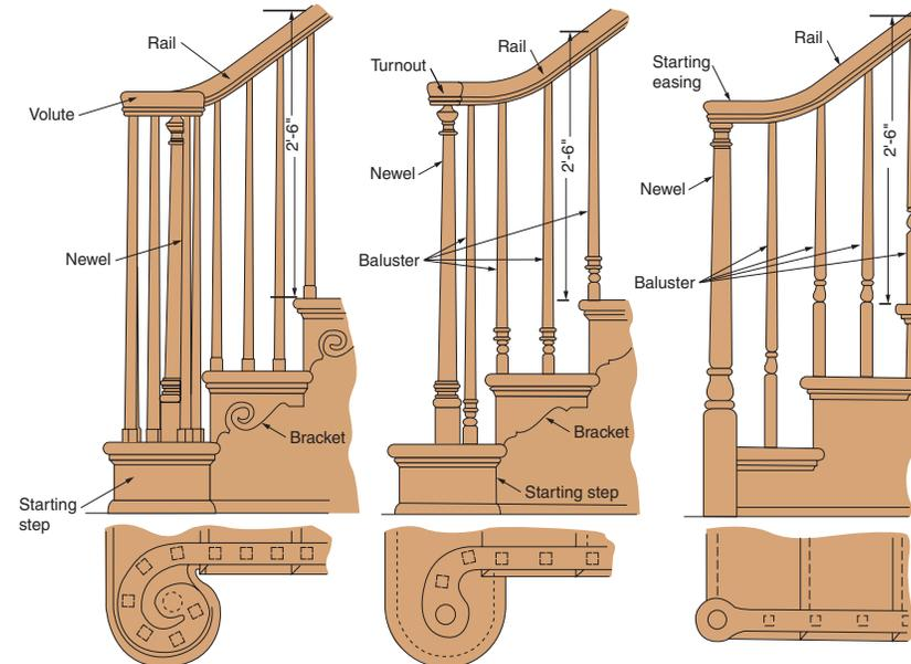
**Figure 18-29.** Balustrade assemblies produced from stock parts. (Colonial Stair and Woodwork Co.)
