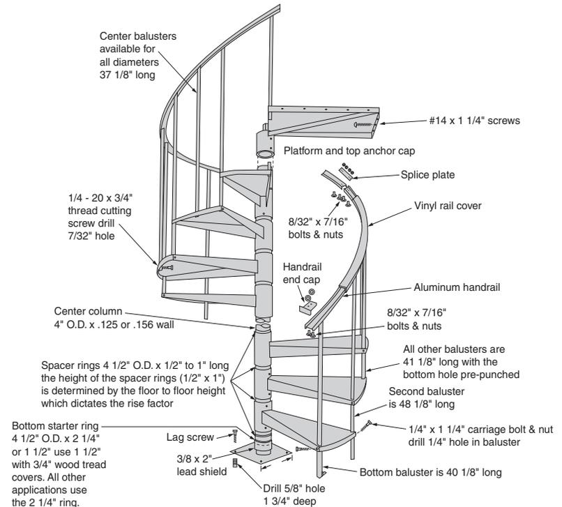
**Figure 18-31.** Assembly drawing of a spiral stairway.
