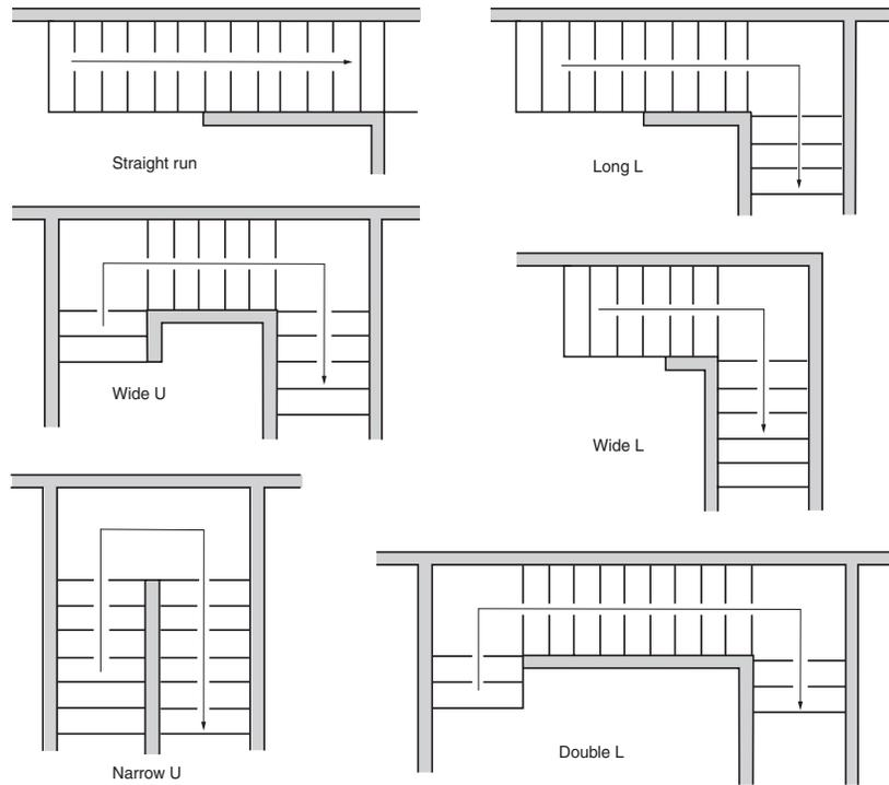
Figure 18-3. Terms used to define various stair types.
