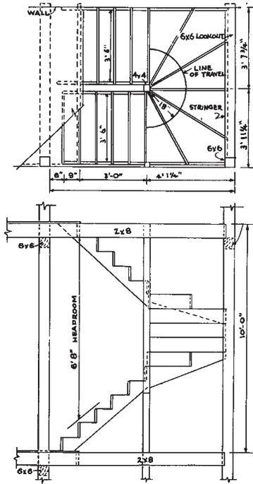
**Figure 18-22.** Typical drawing of a winder stairs. The tread width on the winding section should be the same at line of travel (near middle of stairs) as the tread in the straight run.
