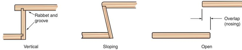
Figure 18-17. Basic stair riser shapes. For the open riser, the tread should overlap the riser at least 2".
