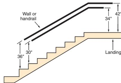
Figure 18-11. A handrail height of 30" at the rake (slope) and 34" at the landings has been an accepted standard. Recently, building codes in some places have been adopting heights of 36" at the rake and 42" at landings. (C-E Morgan)
