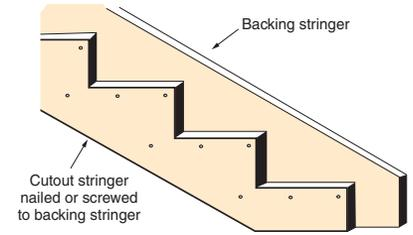
Figure 18-20. This is a semihoused stringer, an adaptation of the cut-out stringer.
