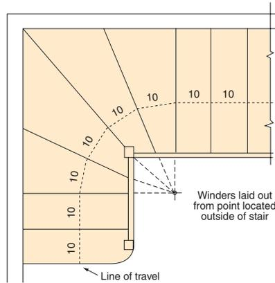
**Figure 18-23.** Laying out a winder stairs with lines representing the tread nosings converging outside of the construction.
