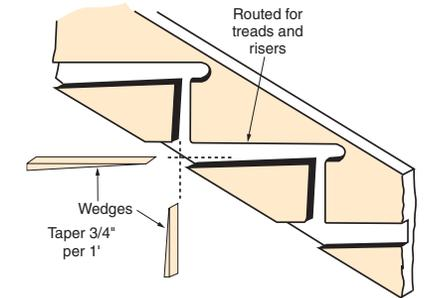
Figure 18-21. In a housed stringer, risers and treads are let into the stringer. This type of housing is difficult to make.
