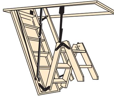
**Figure 18-32.** This disappearing stair unit is designed to fold into the ceiling. The ceiling opening should be framed as the ceiling joists are installed. (Rock Island Millwork)
