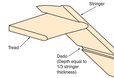
Figure 18-19. Open riser stairs. Treads are set into dados cut in the stringer.
