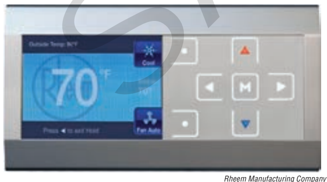
Figure 23-24. A typical electronic wall thermostat with an LCD screen that displays indoor temperature, outdoor temperature, and heating or cooling mode. The thermostat can be used to raise the temperature, lower the temperature, take indoor and outdoor temperature readings, select heating or cooling mode, and select continuous or automatic fan operation.
