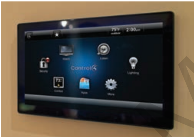
Figure 23-11. A power-stealing thermostat with a touch screen interface. Note this unit is a whole home management system.
