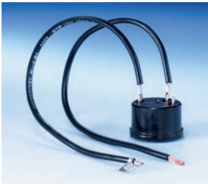
Figure 9-11. This thermal overload is mounted to the shell of a compressor. It is connected in series with the compressor's common wire and opens the circuit when it senses dangerously high temperature.
