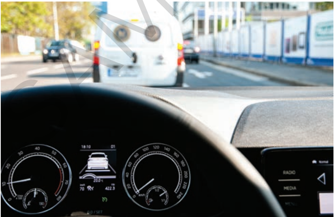
Figure 6-1. Adaptive cruise control in use. The following distance is reflected on the vehicle's dashboard.
