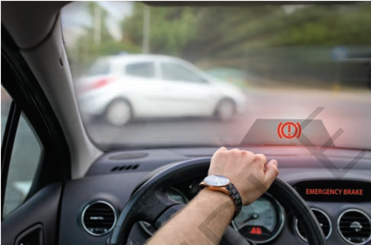
Figure 6-13. The vehicle's AEB system helps it brake to avoid a collision.
