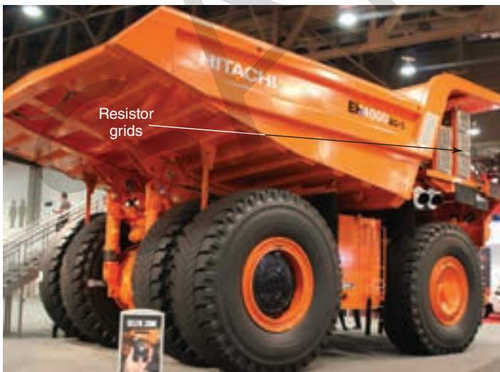
Figure 26-29. This Hitachi EH 4000 AC 3 electric-drive haul truck has a 243-ton payload capacity. Its resistor grid boxes dissipate energy during braking and are visible above the engine's exhaust, just right of the operator's cab.
