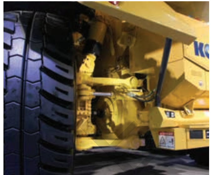
Figure 26-33. The Komatsu four-wheel drive, four-wheel steer truck does not have an operator's cab. A—A photo of the back of the truck. Without an operator's station and with four-wheel steer, the truck drives the same in forward and reverse. B—A close-up view of the steerable drive wheel.
