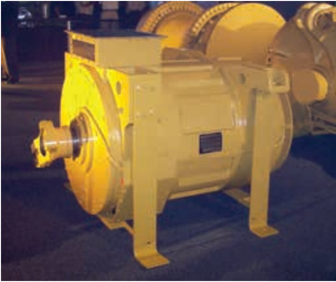
Figure 26-24. An 795F AC generator is located at the rear of the truck and is driven by the engine through an isolation coupler (damper assembly) and drive shaft.
