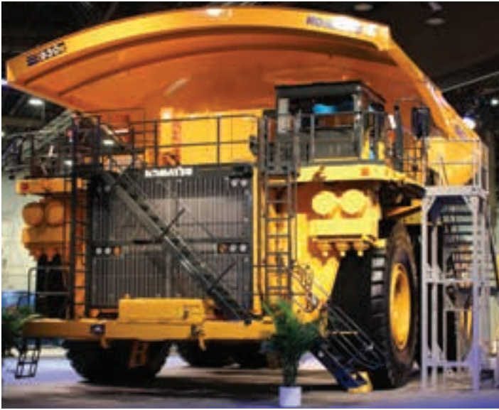
Figure 26-31. The Komatsu 930E electric-drive truck uses GE's AC electric drive. The AC control cabinet is located beside the operator's cab.
