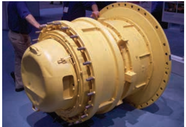
Figure 26-1. This GE 772E DC electric drive motor was used to propel an electric-drive haul truck.
