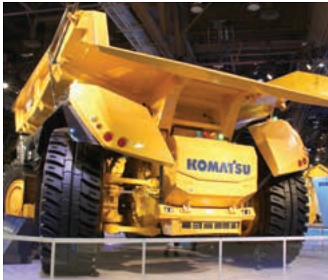
Figure 26-33. The Komatsu four-wheel drive, four-wheel steer truck does not have an operator's cab. A—A photo of the back of the truck. Without an operator's station and with four-wheel steer, the truck drives the same in forward and reverse. B—A close-up view of the steerable drive wheel.
