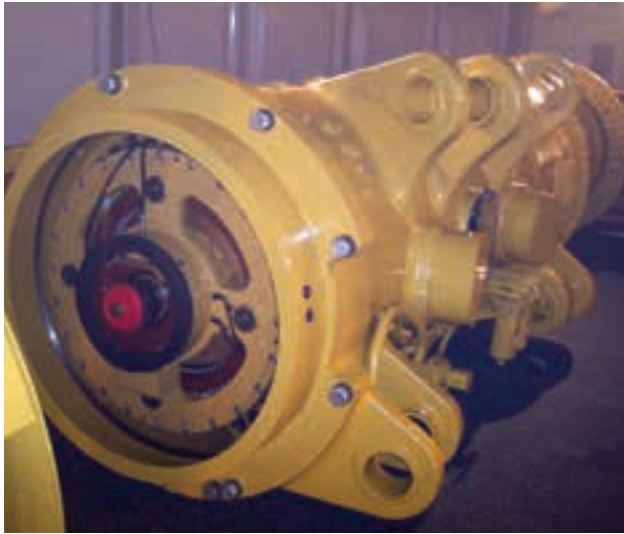
Figure 26-27. A Caterpillar 795F AC truck has two AC induction motors in the truck's axle housing.
