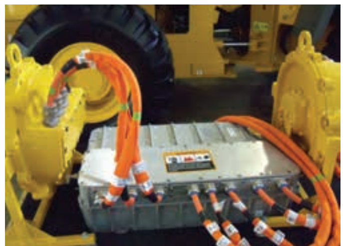
Figure 26-39. An early version of the 644K inverter. The loader's inverter is liquid-cooled. The inverter controls the AC electric motor.
