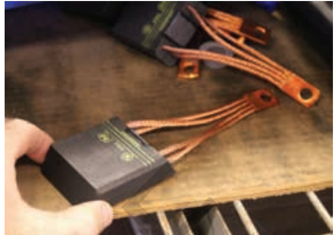
Figure 26-12. This brush is used in a locomotive's DC traction motor.
