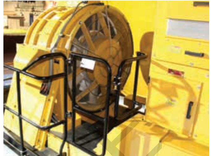
Figure 26-28. The radial grid acts like a brake resistor. It is located beside the control power inverter cabinet and has its own cooling fan.
