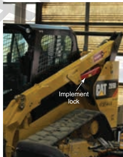
Figure 1-18. Loaders commonly have an implement lock. A—Notice the loader frame is in a lowered position and the red implement lock is in its stored position. B—The implement lock has been placed over the loader's lift cylinder rod and is preventing the loader from lowering.
