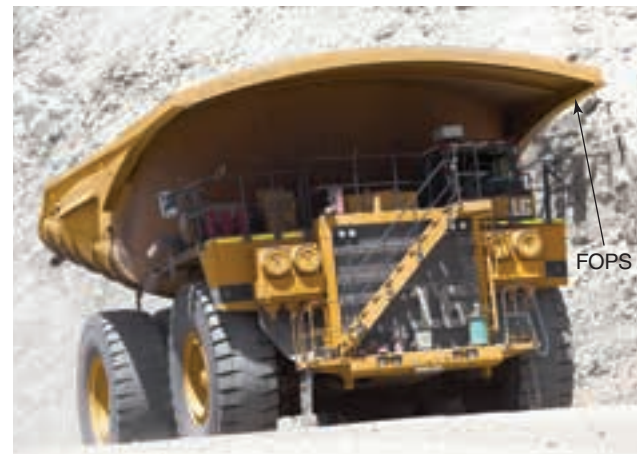
Figure 1-24. The truck bed serves as the FOPS in a rigid haul truck application.
