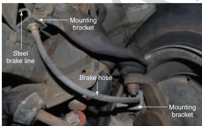
Figure 24-27. Flexible brake hose. The hose connects the steel brake line to the wheel brake assembly.
