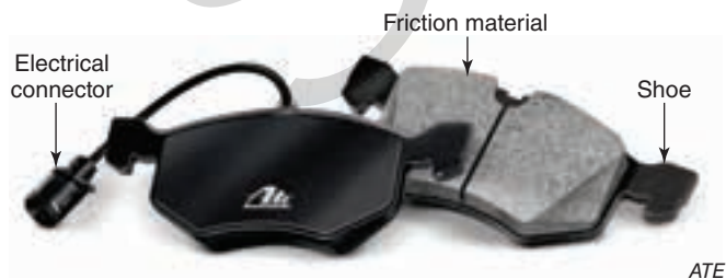
Figure 24-37. This pad wear indicator alerts the driver of worn pads by illuminating a warning light on the instrument panel. Note the electrical connector.
