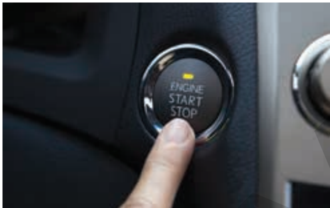
Figure 17-40. The start button on this vehicle is located on the instrument panel to the right of the steering wheel. On some vehicles, the button can be removed to uncover a standard ignition switch for starting the vehicle if the push button system fails.
