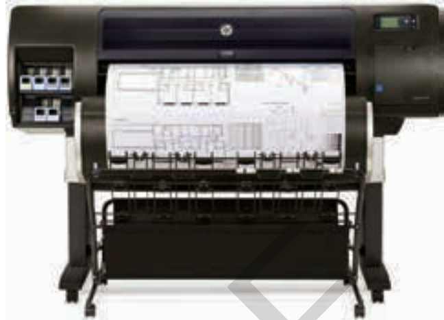
Figure 1-11. High-quality prints can be made from CADD drawings using a printing device such as this large-format inkjet printer.
