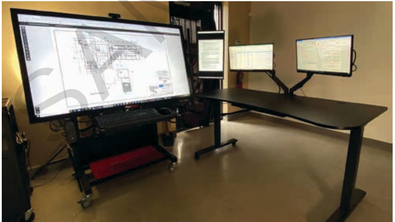
Figure 1-13. This wide-format display table has a large touchscreen monitor and is equipped with three smaller monitors for additional display.
