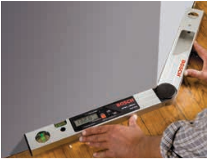
Figure 48-30. A digital angle protractor can measure to within 0.1 degree.
