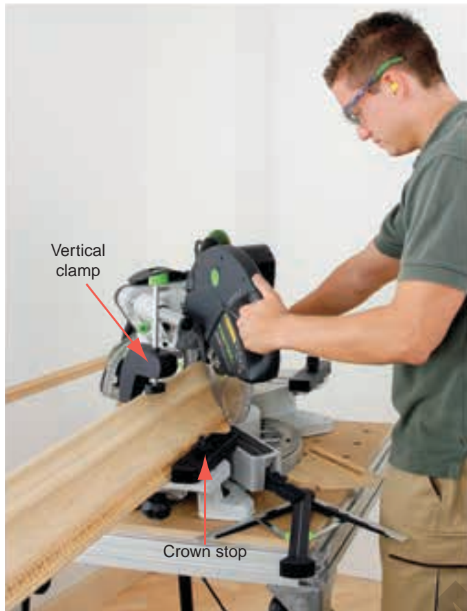
Figure 48-26. This saw is equipped with a crown stop and vertical clamp to position and hold the moulding while cutting.
