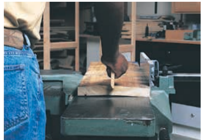
Figure 25-8. The concave side of a cupped face should be placed down.
