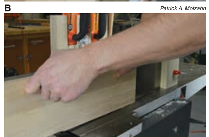
Figure 25-16. Full-length tapers can be done using a jointer. The maximum amount of material to be removed should not exceed 3/8" (10 mm). A—The board is lowered onto the spinning cutter. It must rest a minimum of 1/8" (3 mm) on the outfeed. B—A stop block is securely fastened to the fence to avoid kickback. C—Move the board forward, maintaining pressure on the infeed side until enough of the board is on the outfeed bed to avoid tipping the stock.
