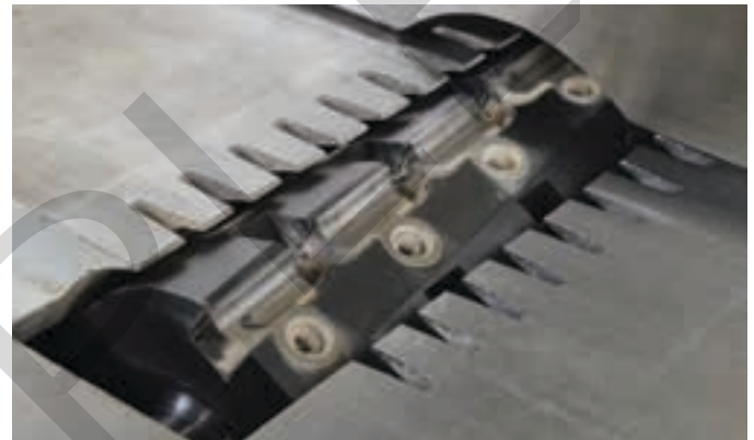
Figure 25-29. These self-locating, carbide inserts can be changed easily by loosening the set screw.
