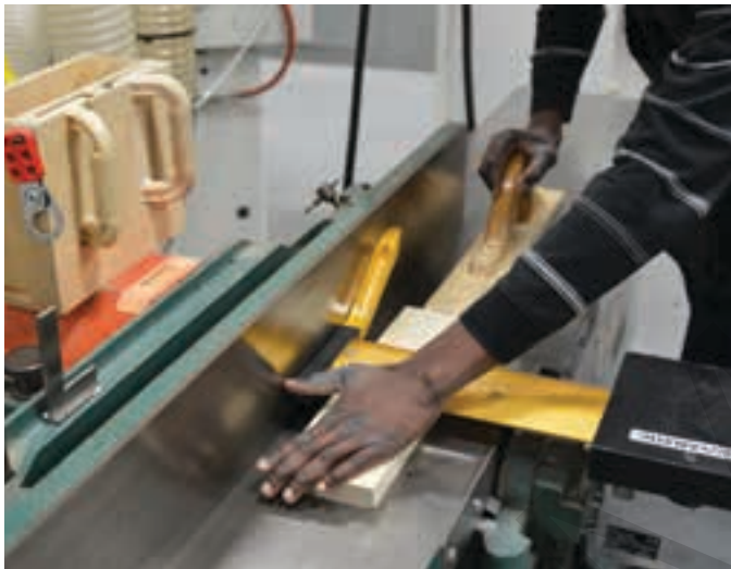
Figure 25-4. A—Swing-type guard. B—Bridge-style guard.
