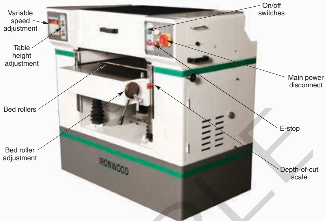
Figure 25-19. Exterior components of a planer.
