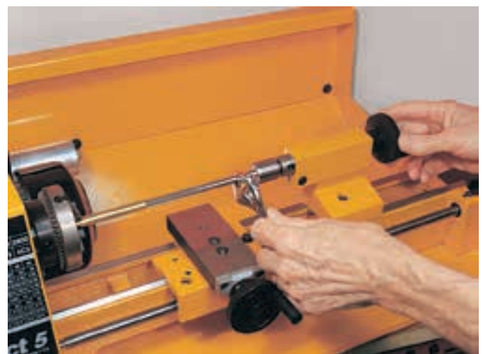
Figure 15-13. Using a hand reamer on the lathe. Never turn on the power when performing hand reaming operations.
