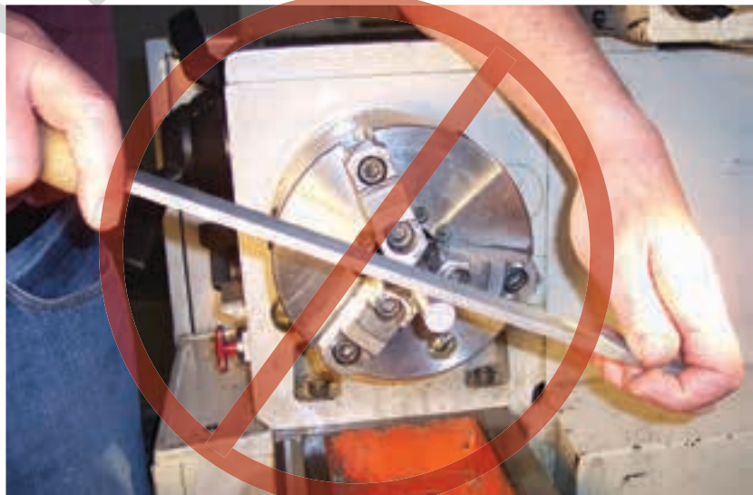
Figure 15-21. A—The left-hand method of filing on the lathe is preferred. B—Avoid using the right-hand method as shown here. Notice that the machinist's left hand and arm are extended over the revolving chuck, which can cause injury.
