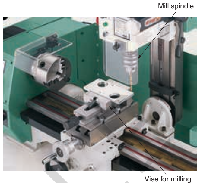
Figure 15-37. Milling attachments on a lathe. A—A lathe with a milling attachment mounted on the back of the bed. B—Workholding devices are fitted on the cross-slide.
