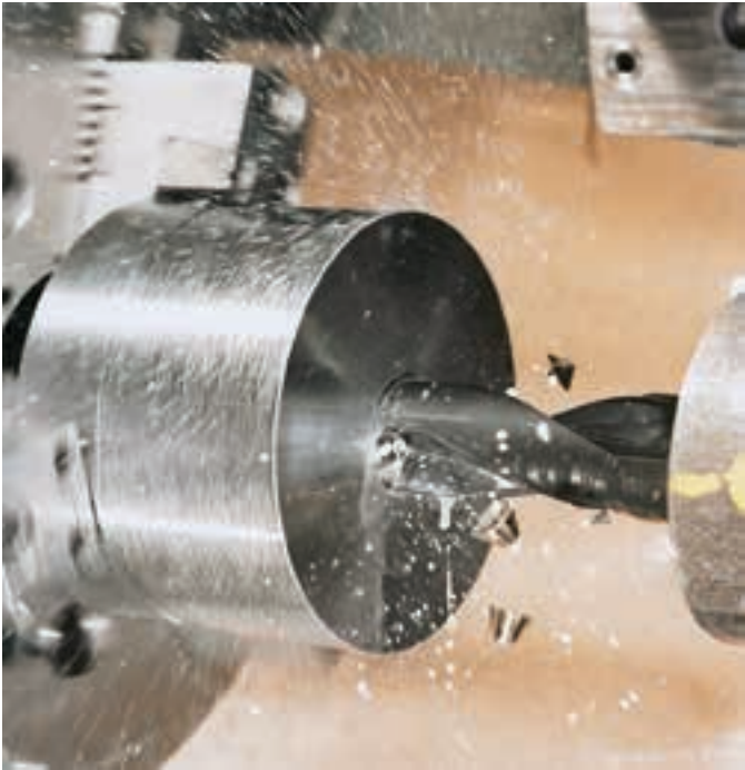
Figure 15-6. When drilling on a lathe, the workpiece is held in the headstock and rotated while the stationary drill, held in the tailstock, is advanced into the work. The cutting fluid helps to reduce heat and flush away chips.
