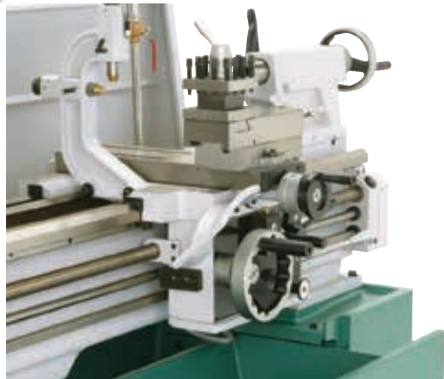
Figure 15-27. A follower rest is used to support long slender workpieces during machining operations.
