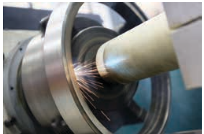
Figure 15-30. A tool post grinder used for internal grinding on a lathe.
