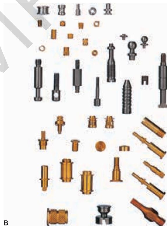
Figure 15-42. Swiss-type automatic turning center. A—This high-precision turning center machines small parts from bar stock ranging from 1 mm to 10 mm in diameter at high production rates. B—These tiny components, produced by a Swiss-type automatic turning center, are used in precision instruments.
