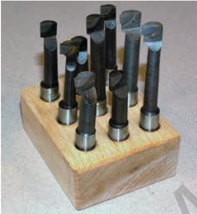
Figure 15-3. A set of carbide-tipped boring bars with 1/2" (12.5 mm) diameter shanks.
