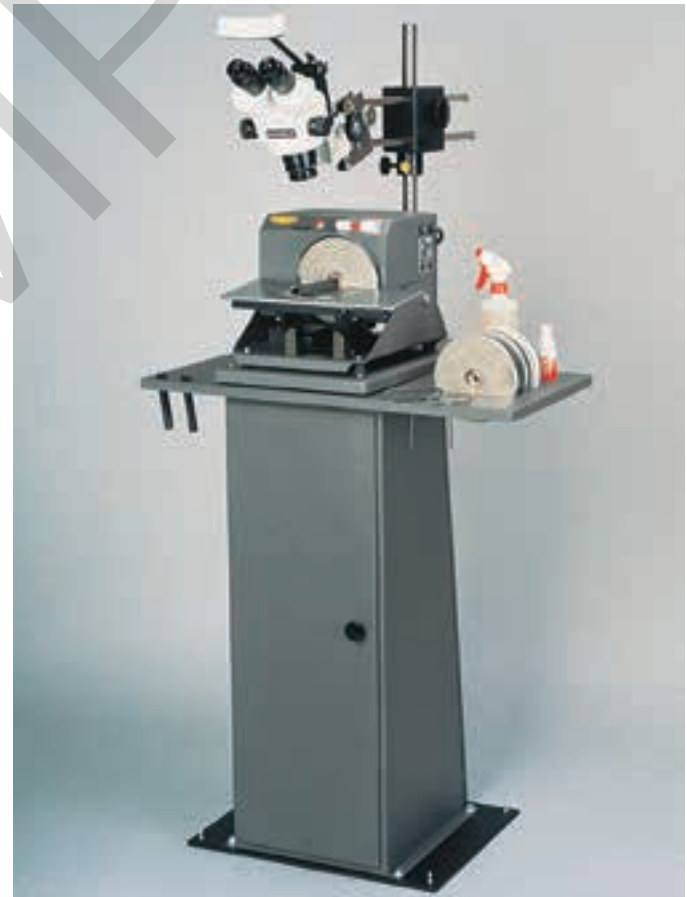
Figure 14-52. A grinder designed for sharpening carbide, cermet, cubic boron nitride, and polycrystalline diamond (PCD) cutting tools. It uses diamond-charged wheels and is fitted with a microscope inspection system.
