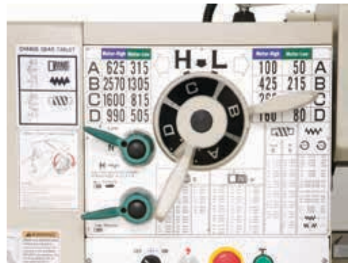
Figure 14-5. Spindle speed control. Speed is increased or decreased by shifting to different gear ratios. On this machine, the desired speed is dialed in.
