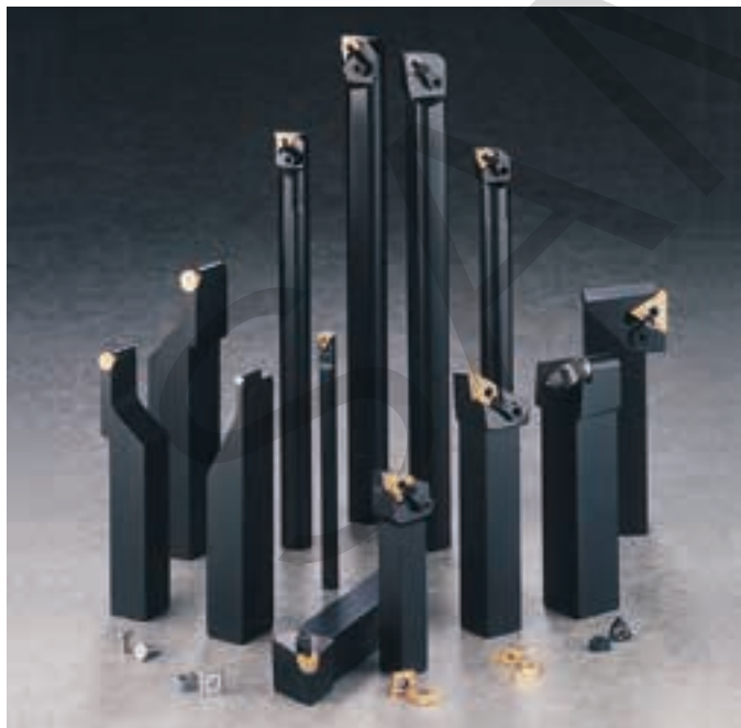
Figure 14-57. A selection of typical toolholders and replaceable carbide insert cutting tools for the lathe. Each insert has three or four cutting tips. The inserts are clamped in place on the holder and can be indexed (rotated into position) to present a new tip when the one in use becomes dull.
