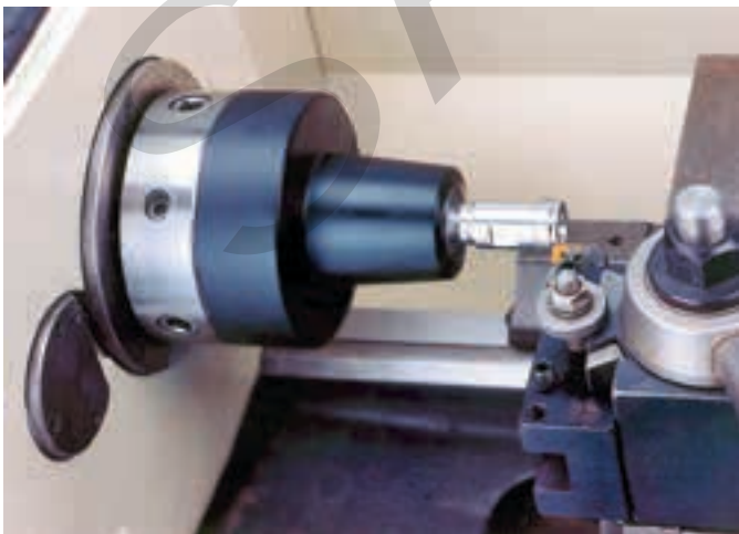
Figure 14-40. A draw-in collet chuck.
