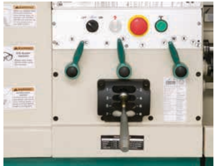
Figure 14-13. A quick-change gearbox for cutting both inch and metric size threads.
