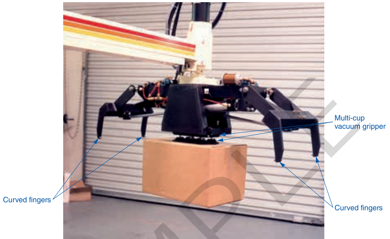
Figure 9-9. When an object with large surface area must be grasped, a multi-cup vacuum gripper is often used. The gripper pictured also has curved fingers to provide additional support when moving large objects.
