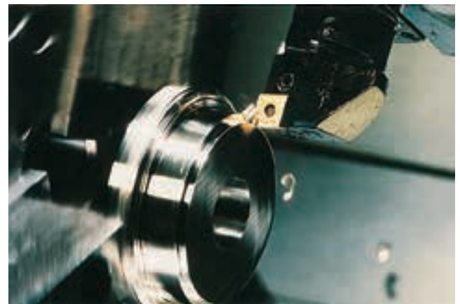
Figure 10-18. Machine tools and operations used to produce hole features. A—A cutting tool with a drill bit. B—A cutting tool with a reamer bit. Reaming produces a very accurately sized hole. The hole is first drilled slightly undersize before reaming. C—Countersinking prepares a hole to receive a flathead screw. D—Boring is an internal machining operation. E—Turning work on a lathe.
