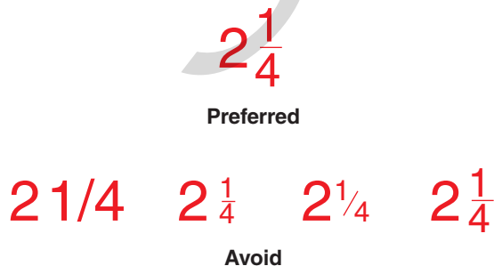
Figure 10-16. Numerals and fractions must be drawn to the proper size and orientation.
