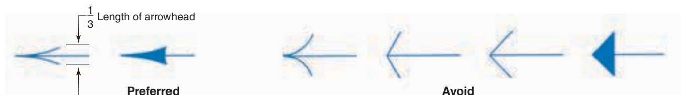
Figure 10-6. Arrowheads are drawn 1/8" long. The solid arrowhead is generally preferred.
