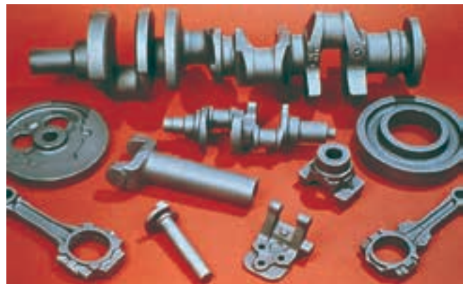
Figure 10-17. These automobile castings are typical of manufactured parts that contain circles, round holes, and arcs in their design.
