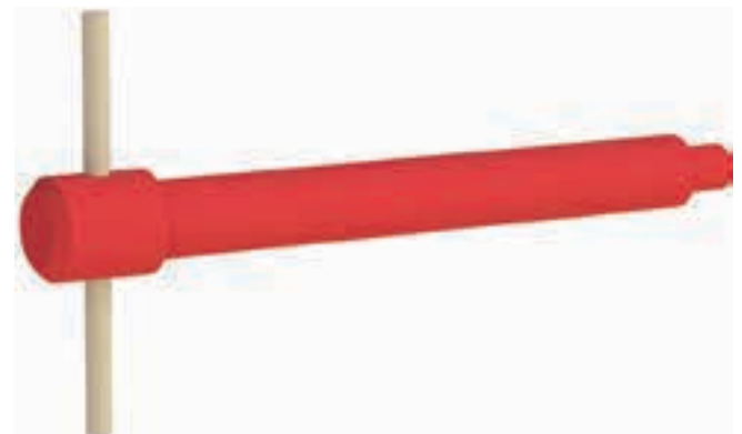
Figure 7-32. A subassembly consists of two or more parts. This subassembly is made up of two parts, a screw body and a pin, and is used in an assembly of a C-clamp.
