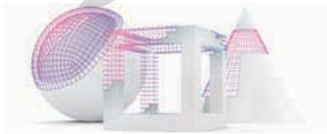
Figure 7-24. A surface model is a representation of the outer “skin” of the various surfaces simulating the object.
