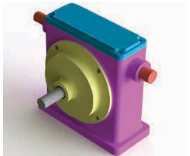
Figure 7-25. Parametric modeling programs provide powerful modeling tools that allow object dimensions to be changed throughout the modeling process. Any changes made affect the entire model.
