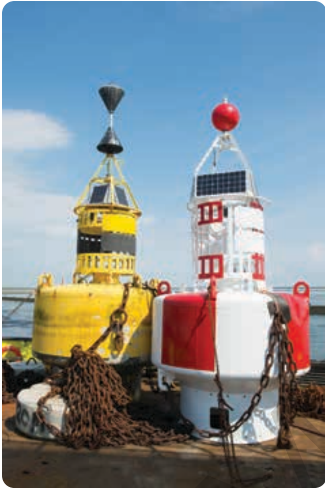
Figure 11-8. Solar cells can be used to power several different types of devices, such as a navigational buoy. What are the benefits and limitations of generating electricity from solar cells?
