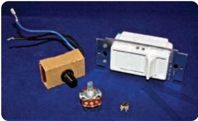
Figure 11-16. Goodheart-Willcox Publisher These are common variable resistors. What are a few variable resistors you commonly encounter in buildings, in vehicles, or on devices?
