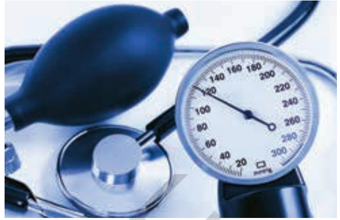
Figure 10.30 Each long line on the manometer gauge represents 10 mmHg. What pressure measurement is shown on this gauge?
