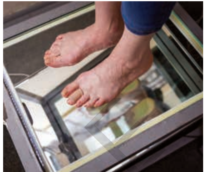
Figure 4.44 Orthotists may use a digital foot scan to provide the basis for custom shoe insoles.
