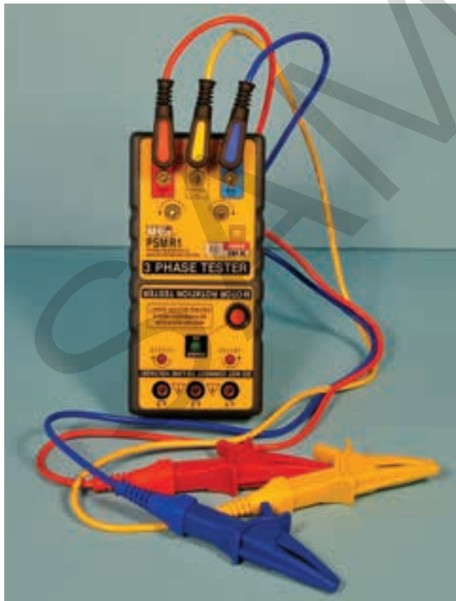
Figure 20-28. A phase sequence and motor rotation tester is a relatively simple and valuable testing device.
