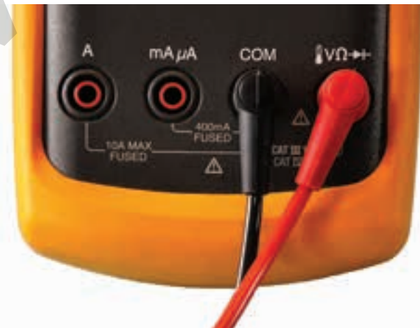
Figure 20-12. A digital multimeter with the test leads appropriately connected to measure voltage or resistance. Note the two current jacks to the left of the test leads.
