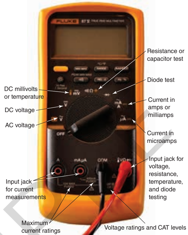
Figure 20-11. Most digital multimeters (DMMs) have features similar to those shown here.
