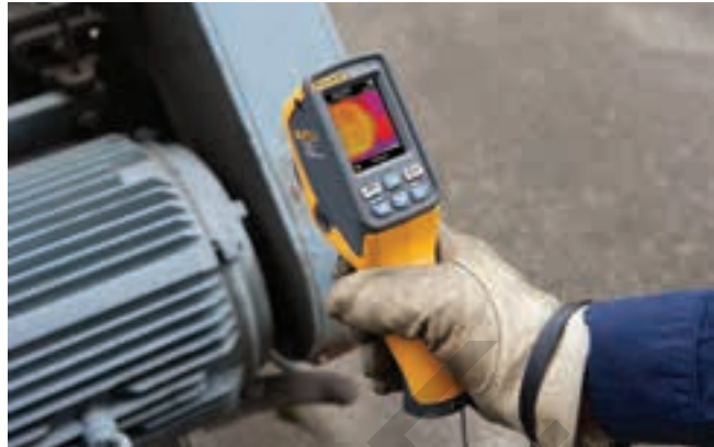
Figure 20-29. Infrared (IR) thermometers determine temperature by measuring the amount of infrared radiation emitted from an object.
