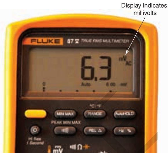
Figure 20-16. A DMM displaying a phantom voltage. Be careful in interpreting the reading. Notice the mV indication in the display. The reading is 6.3 mV, not 6.3 V.
