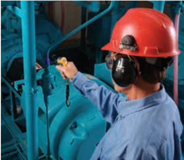
Figure 20-2. Always wear the appropriate personal protective equipment (PPE). This industrial maintenance technician is wearing hearing protection, safety glasses, and a hard hat while taking temperature measurements.
