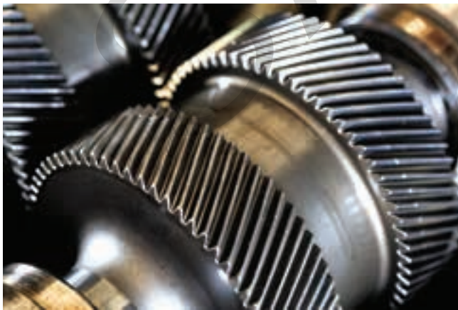
Figure 12-27. A double helical gear is manufactured on the same hub, with a space between the sets of teeth.
