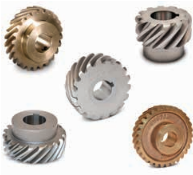
Figure 12-26. The angle of helical gear teeth allows several teeth to engage at the same time.
