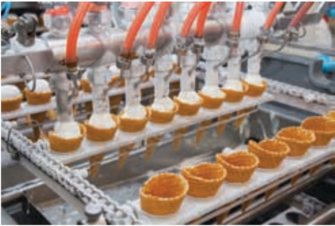
Figure 1-28. Have you ever thought about how specialized agricultural machinery must be? This is just one example of a specialized machine, which fills ice cream cones for individually frozen treats.
