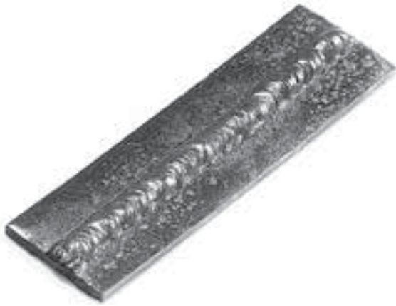
Figure 14-5. A good example of running a bead with filler metal. Note the straightness, good penetration, and uniform bead size and shape.
