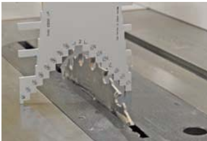
Figure 23-10. Blade height is set easily with this gauge.
