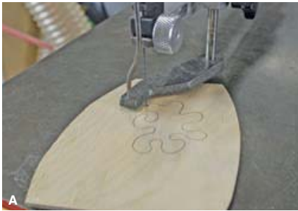
Figure 23-56. When cutting interior curves, free the top end of the blade and thread it through a predrilled hole.
