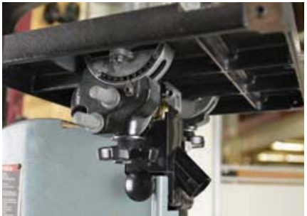
Figure 23-49. Adjust the table angle by loosening the trunnion knobs and using the tilt scale or a bevel to set the angle.
