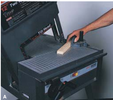
Figure 23-50. Beveling on the band saw. A—A tilting head and a miter gauge is used to produce a compound bevel. B—A tilting table with or without a fence may be used for straight bevel.
