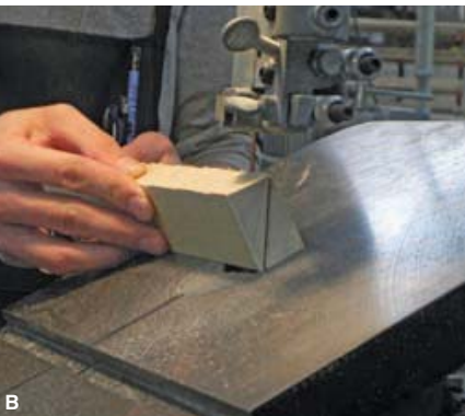
Figure 23-50. Beveling on the band saw. A—A tilting head and a miter gauge is used to produce a compound bevel. B—A tilting table with or without a fence may be used for straight bevel.
