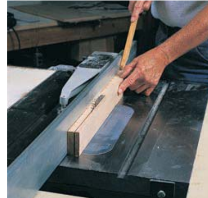
Figure 23-21. A one-pass resawing operation. Use push sticks to feed the material as your hand nears the blade. Guards are removed to show procedure.
