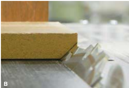
Figure 23-19. When beveling, feed stock so the excess falls off below the blade. Guards have been removed to show the operation. A—Ripping. B—Crosscutting.
