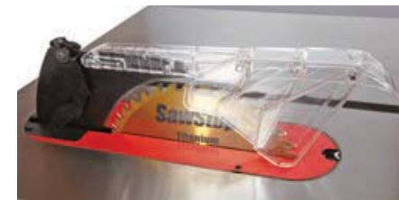
Figure 23-4. This blade guard is mounted to the saw trunnion under the table.
