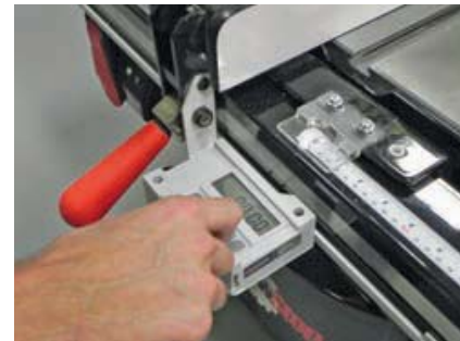
Figure 23-2. A rip scale may be supplemented with a digital readout (DRO).
