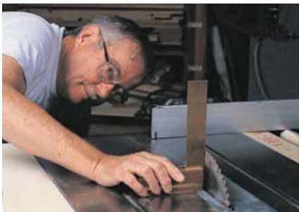
Figure 23-11. Check to ensure the blade is at 90° to the table. Avoid placing the square against the saw teeth.
