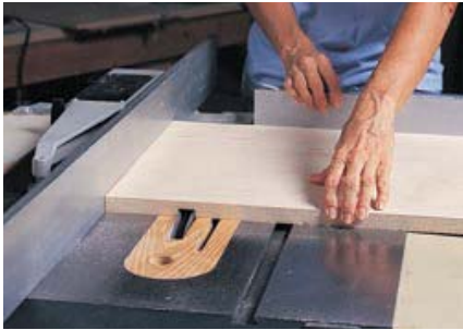
Figure 23-9. Both the rip fence and miter gauge may be used for cuts that do not go completely through the material. A dado cut is shown. The guard has been removed to show this operation.
