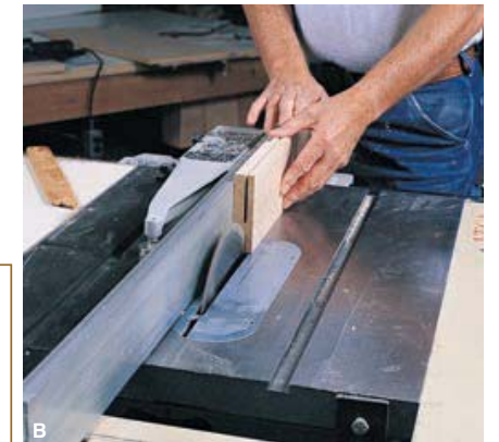
Figure 23-22. A two-pass resawing operation. A—Set the blade height just over half the material width. Keep the same surface against the fence for both passes. B—Use push sticks to feed the material as your hand nears the blade.
