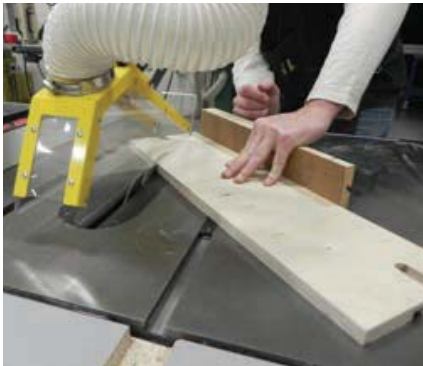
Figure 23-20. Sawing a miter.
