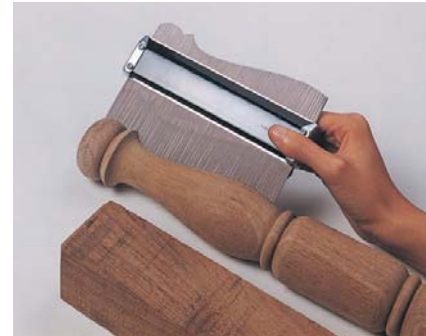
Figure 12-27. A profile gauge conforms to the shape of the piece to be copied.
