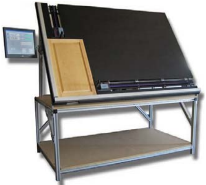
Figure 12-37. This measurement table is used to check and record panel measurements. These can be uploaded to a computer.
