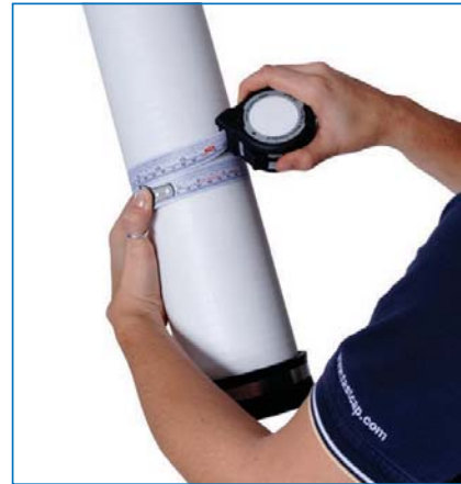
Figure 12-8. Two types of tape measures. The bottom tape measure is extra flexible to allow for measuring curved surfaces.
