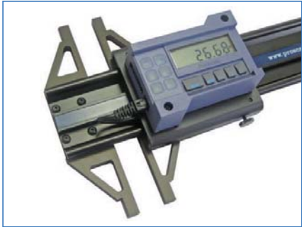
Figure 12-36. Digital measuring tools are capable of recording inside, outside, diagonal, hole-edge and hole-hole dimensional measurements.
