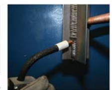
Figure 18-9 The suggested gun angles for welding a multiple-pass fillet weld on a T-joint in the vertical position. Notice that the work angle must change slightly from 45° for the second and third passes.
