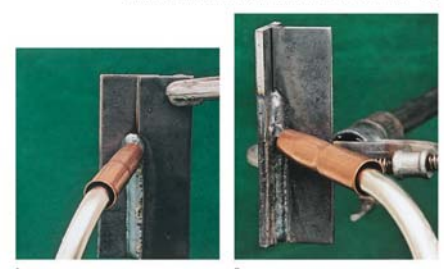
Figure 18-8 A—A fillet weld being made on a vertical lap joint. This weld is being made uphill using the forehand welding method. B—A fillet weld being made on a vertical T-joint. The weld is being made uphill using the forehand welding method.
