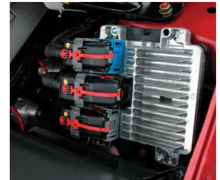
Figure 7-3. The ECM in this vehicle operates all of the vehicle systems, either directly or by controlling messages to other vehicle computers. Fins are cast into the body for heat removal.
