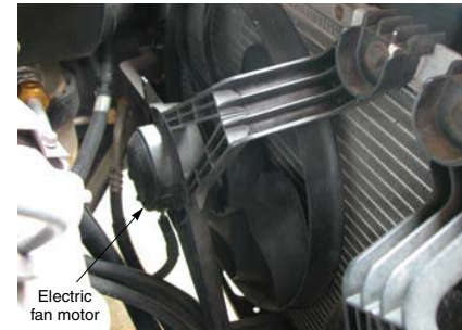
Figure 7-30. Electric cooling fans can be controlled by the ECM. The ECM can turn the fan on and off and determine whether it runs at high or low speed.
