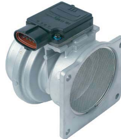
Figure 7-12. Mass airflow sensors (MAF) are installed in the air intake duct between the air filter and throttle valve. (Cardone)
