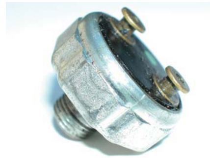
Figure 7-24. Pressure switches such as this one are installed on the case or valve body of automatic transmissions/transaxles to sense internal fluid pressure. When hydraulic pressure applies a band or clutch, the fluid pressure also activates the pressure switch. This signals the ECM that a shift has taken place.
