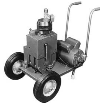
Figure 11-27. Two-stage vacuum pumps are available in different sizes for varying applications. A—Small 1.6 cfm pump. (Thermal Engineering) B—Cart-mounted 15 cfm unit for use on large systems. (Robnair Mfg. Corp.)
