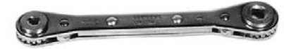
Figure 11-9. The most popular type of service valve wrench is a ratchet-type. It has four sizes of openings and is easily reversed. (Robinair Mfg. Corp.)
