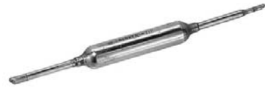
Figure 11-35. Small filter-drier intended for a domestic unit. The copper tubes at each end are brazed into the system at the condenser outlet. (Parker-Hannifin)
