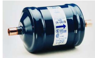
Figure 11-32. This filter-drier is designed for attachment to the liquid line with flare fittings. Other types are designed for brazing into the line. Note the arrow indicating the proper direction of refrigerant flow through the device. To keep the desiccant at full effectiveness, the seal caps on the fittings should be left in place until just before the filter-drier is installed. (Alco)
