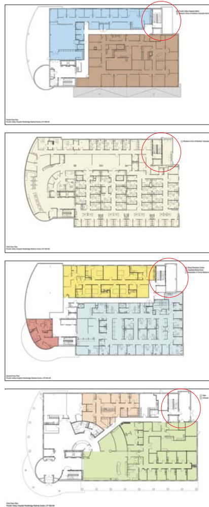
Figure 14-35 Block and stack diagrams are essential to evaluate alignment of building features such as stairways and elevators in all levels of a building. Note the circled areas on these drawings are a key area the designer must evaluate for egress and circulation.
