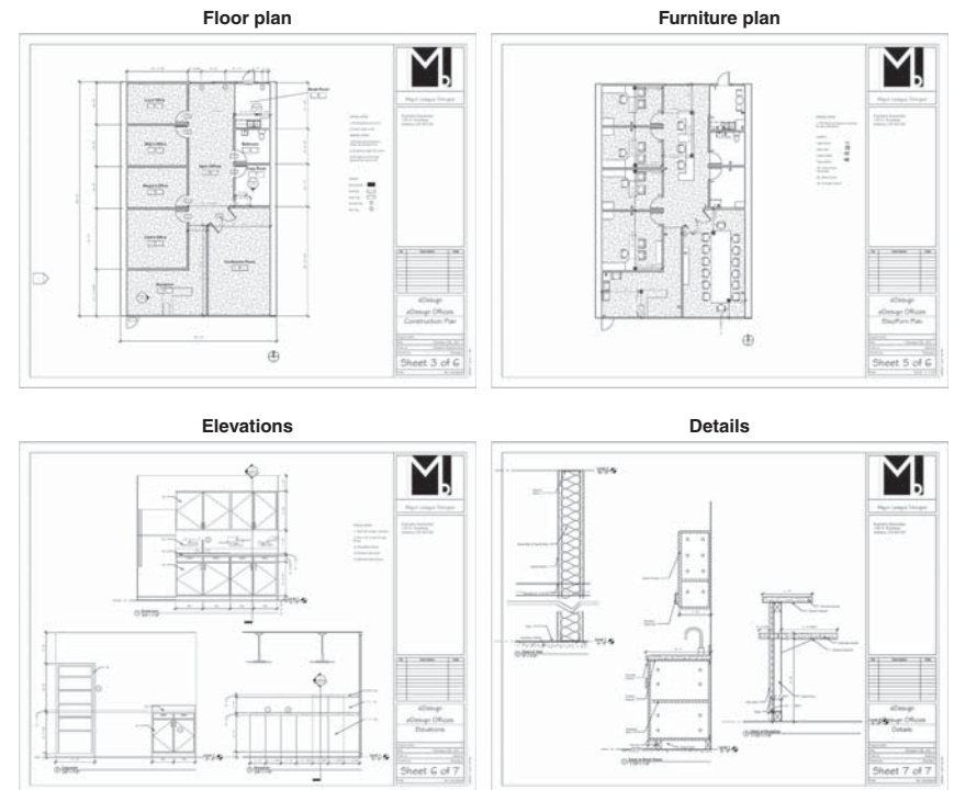
Figure 14-37 Contract documents contain the working drawings and specifications needed for construction.
