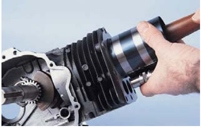
Figure 19-13. A ring compressor is used to squeeze the ring ends together while the piston is pushed into the cylinder.
