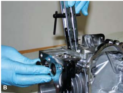
Figure 19-2. Compress the valve springs and install the keepers. A—When using an L-head type compressor, place the retainers on the spring and then compress the assembly. B—Place the spring and retainers into position and then insert the valve stem through them. Reposition the retainer so it locks on the valve stem, and then open the valve spring compressor.
