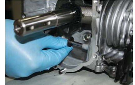
Figure 19-5. Tilt the engine so the valve lifters will not fall out of their guides.
