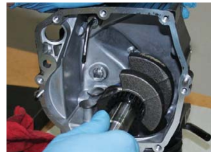
Figure 19-4. Install the crankshaft carefully to avoid damaging bearing surfaces and seals.
