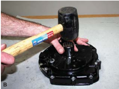
Figure 19-1. Use a seal driver or a socket to tap seals into place. A—Using a seal driver. B—Using a socket.
