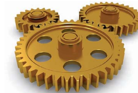
Figure 8-45. On spur gears, the teeth are cut straight across the width of the gears.
