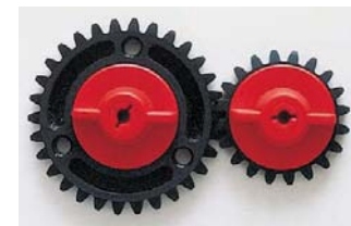
Figure 8-40. Two gears act like levers to convert torque.
