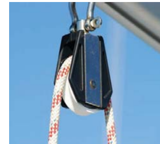
Figure 8-17. A simple pulley changes direction once.
