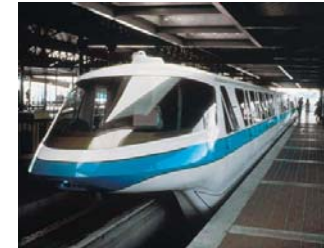
Figure 8-62. One of the effects of streamlining is to reduce air drag, which is a form of friction.
