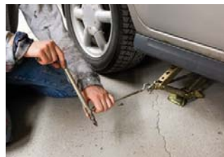
Figure 8-33. A—A scissor jack lifts heavy loads with less effort applied. B—As the screw of the jack is turned, the two ends of the jack are forced to move toward each other, and the car is raised.
