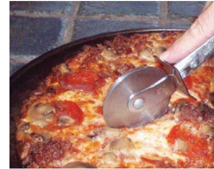
Figure 8-25. A pizza cutter is a form of wheel and axle. Where are the effort, fulcrum, and resistance located?
