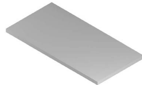
Figure 1-4. The sketch from Figure 1-3 is extruded .25” to create a solid part.
