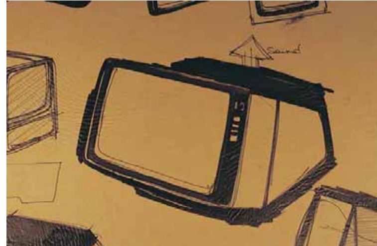
Figure 10-8. In this refined product sketch, the shape has been worked out and shading has been added to improve the looks of the sketch. (RCA)
