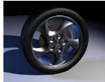
Figure 7-20 A surface model is a representation of the outer “skin” of the various surfaces simulating the object. (Discreet, a division of Autodesk)
