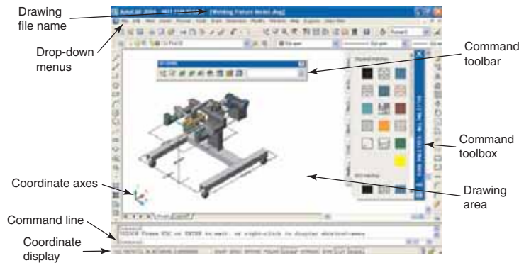
Figure 7-4 The drawing display of a typical CAD program includes drop-down menus, toolbars, and status displays. Commands can be accessed in a variety of ways to suit the user's needs. (Autodesk, Inc.)
