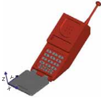
Figure 7-10 A user coordinate system is used to establish a drawing plane in 3D space so that objects can be drawn on the surface of the plane. The XYZ coordinate axes identify the orientation of the drawing plane. In this 3D model of a phone, the XY drawing plane is oriented so that objects can be added to the mouthpiece. Note the direction of the axes.
